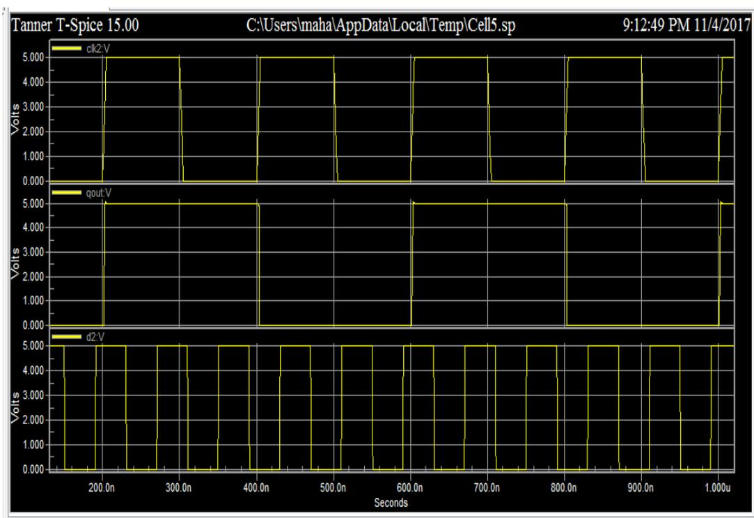
Fig 2: Simulation result of classic master-slave positive-edge-triggered flip-flop
