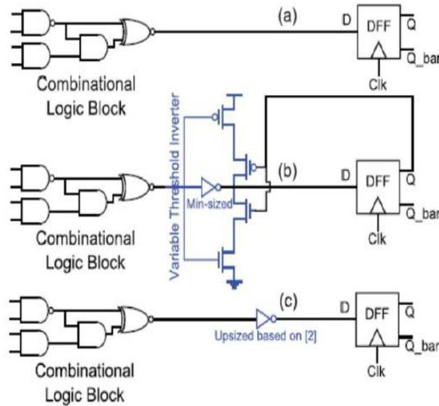
Fig 3: Block diagram of (a) original nonequalized design, (b) equalized design with one feedback path ON, and (c) buffer-inserted nonequalized design.
