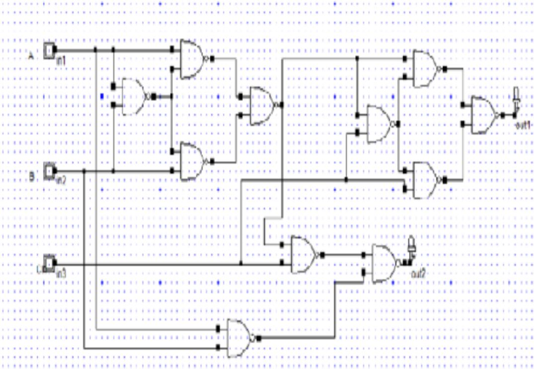
Fig 7: RCA in NAND gate Circuit diagram
