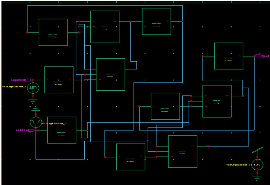
Fig 1: Circuit diagram of classic master-slave positive edge-triggered flip-flop
